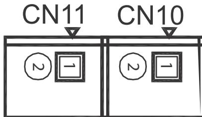
**Figure 1-13: DC 5V and 3.3V Connectors Configuration**
