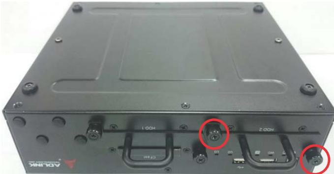
2. Withdraw the HDD rack.
