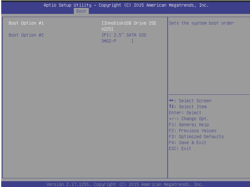
Specifies the priority of boot devices. All installed boot devices are detected during POST and displayed. Target Boot Option # and click to select the desired device.
