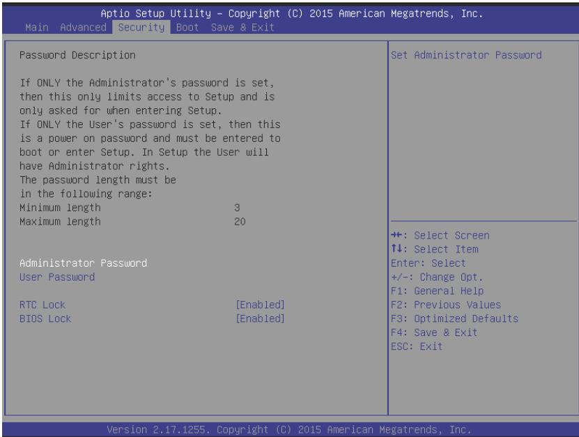
If only the Administrator password is set, access is limited and the password requested on Setup. If User password is set, it acts as a power-on password and must be entered to boot or enter setup. In Setup the user receives
