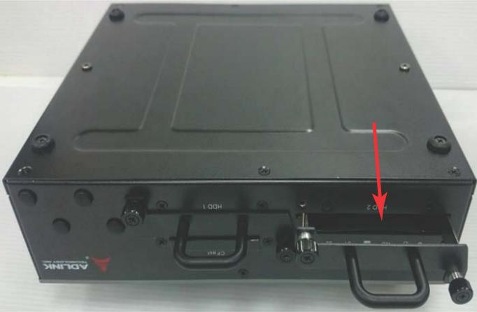
3. Seat the HDD or SSD in the HDD rack.
