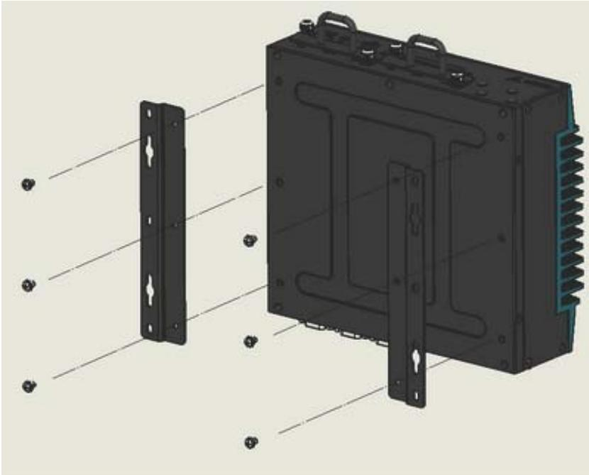
3. Once final assembly is complete, mount the MXE-5500 series controller on the wall via the screw holes.
