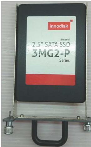
4. Fix the HDD or SSD to the rack using the 4 included M3 screws.
