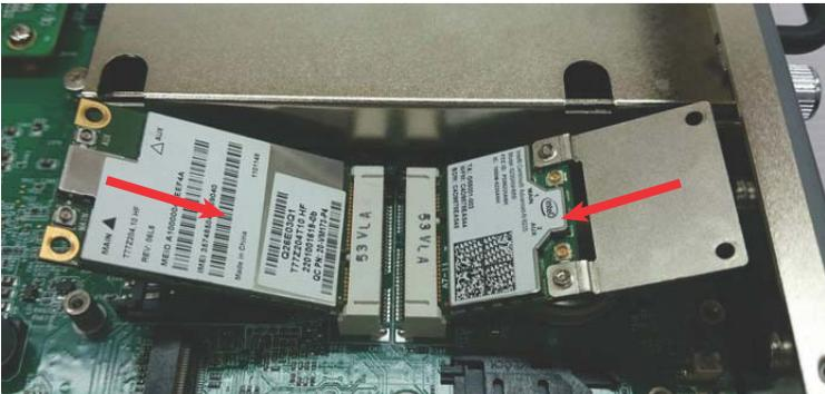
5. Seat the mini-PCI-E wireless module and use the 4 included M2.5-P-head-L5 screws to fix.
