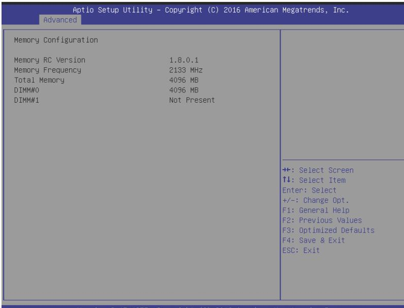
Shows current system Memory RC Version and values for memory frequency, total memory, DIMM#0, and DIMM#1.
