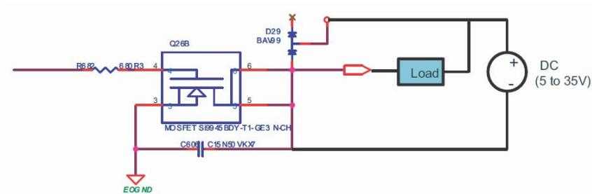
Figure 1-9: Isolated Digital Output Sample Application Circuit
