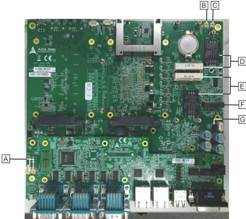
**Figure 1-11: Internal I/O**
