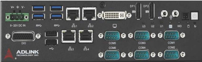
**Figure 1-6: Front Panel I/O**
